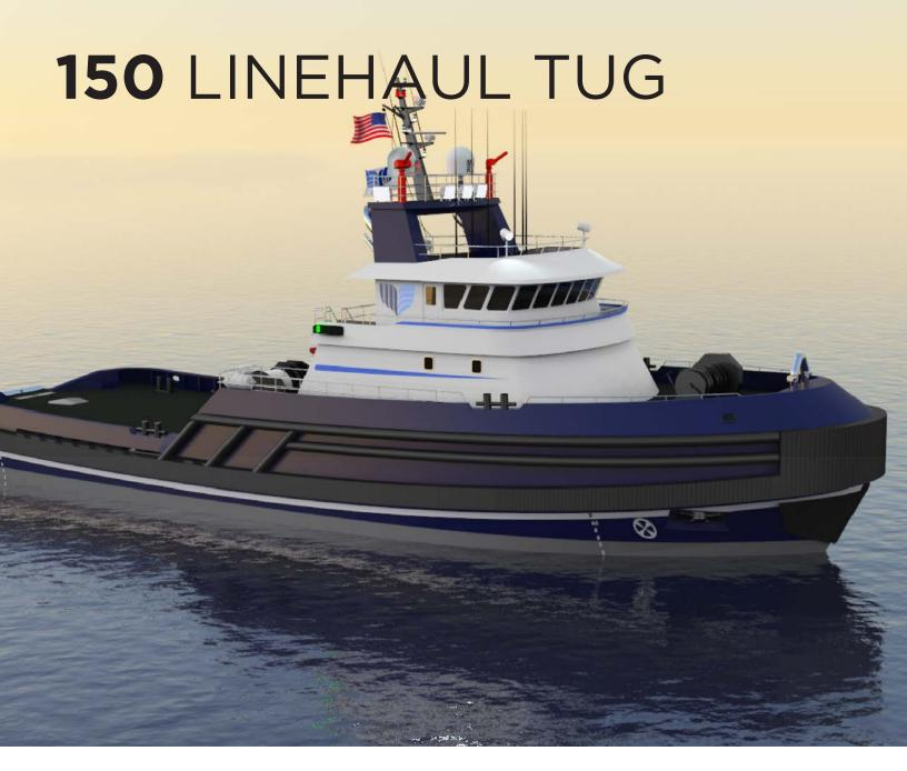
The Jensen 150 Linehaul Tug design is the next generation of state-of-the-art linehaul tugs. The tug features include a baseline Z-drive configuration, Dynamic Position options, an environmental design equipped with a double hull in way of oil tanks, and 360 degree visibility from the wheelhouse. A less obvious yet most desired feature is the special construction techniques designed right into the vessel that reduce both cost and time of construction.
