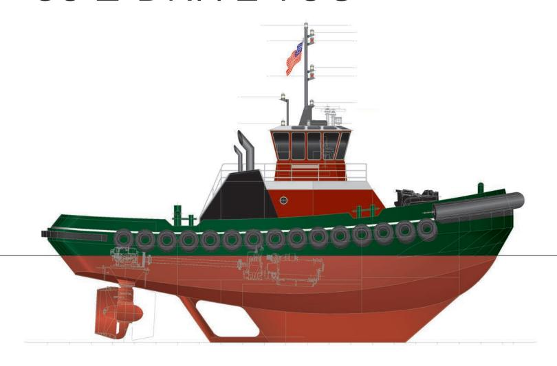
The purpose behind the Jensen 84 Z-Drive Harbor Tug design is to create a maneuverable, powerful, tug to handle most jobs at the lowest operating costs. Its capabilities include ship assist, cargo transportation, coastal towing, and construction operations. The vessel features a wide hull for optimal stability in all operating modes, a forward escort hawser winch and an H-bitt and hydraulic capstan aft for towing, and 360 degree visibility from the wheelhouse.
