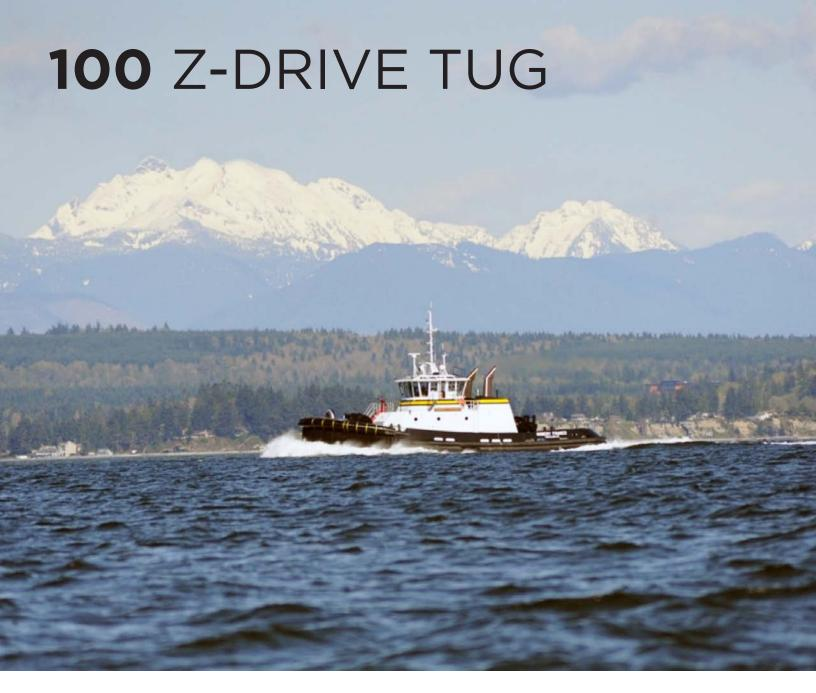
The Jensen 100 Z-Drive Tug design was developed to provide a maneuverable and powerful tug specializing in ship assist and escort work. In addition, the tug also features engines certified for EPA tier 3 operations, a wide hull for stability in all operating modes, a deep skeg forward for escort work, a state-of-the-art escort hawser winch installed forward with a large stainless steel clad staple, and 360 degree visibility from the wheelhouse.
