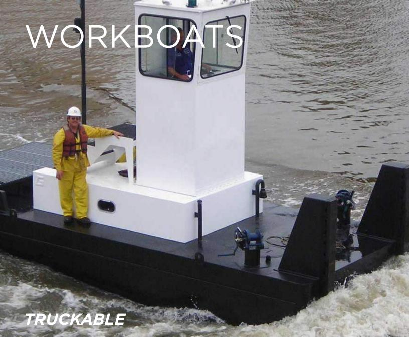
Our "truckable" workboats are ideal for inland lakes and remote locations. The "truckable" units can be of simple design or quite complex ranging from passenger – truck ferries to rail pontoons and crane and spud barges. Great Lakes Shipyard also produces both a single-screw and twin-screw truckable work boat with push knees and collapsible pilothouse.
