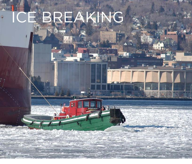
The Great Lakes Towing Company's tugs are available to perform commercial ice breaking services during the winter months of the Great Lakes Navigating season. Our tugs are capable of breaking ice of up to three feet thick and windrows up to six feet high. Normally, we provide ice breaking services within the harbors and in dock areas and slips.
